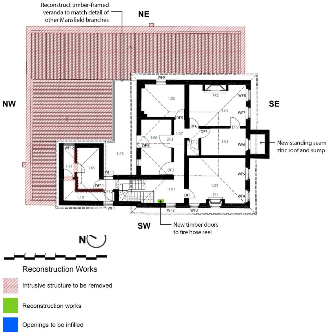
Figure 2 – First Floor Plan (Based on drawing in Tropman and Tropman Heritage Impact Study)
